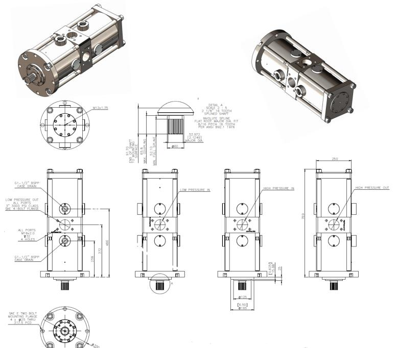
Please note: The rear of the Power centre must be supported on installation.
